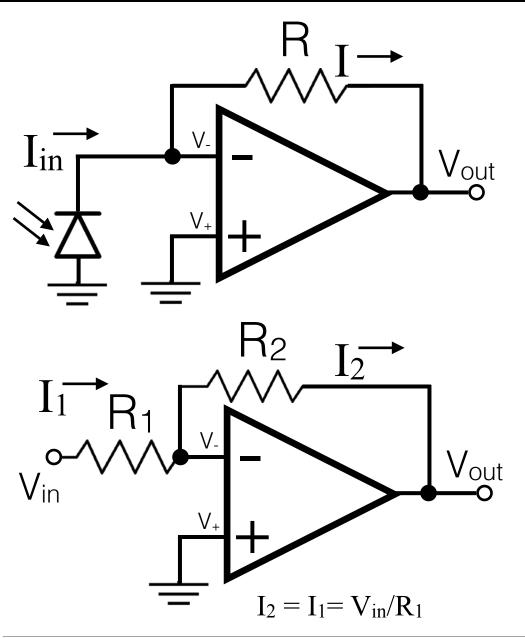
Rule 2 means  $V_-$  = ground. Called a "virtual ground".
