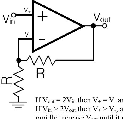
If  $V_{out} = 2V_{in}$  then  $V_+ = V_-$  and there is no difference to amplify, so no change. If  $V_{in} > 2V_{out}$  then  $V_+ > V_-$ , and that positive difference is strongly amplified to rapidly increase  $V_{out}$  until it reaches  $2V_{in}$ .
