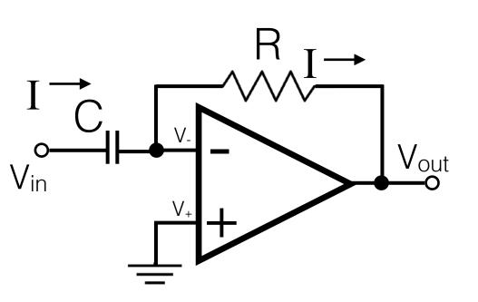
Rule 2 means  $V_-$  = ground. Called a "virtual ground".
