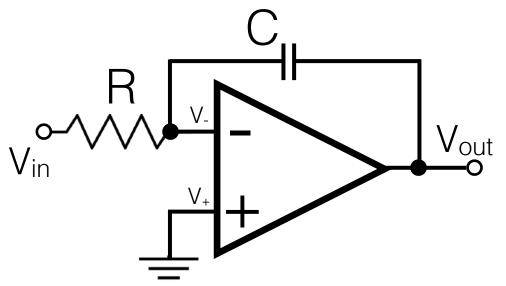
Can also think of this in terms of complex impedance, where it is an inverting amplifier with gain  $G = -X_C/X_R = -(-j/\omega C)/R$  $G = j/\omega RC$ Gain increases for low frequency.
