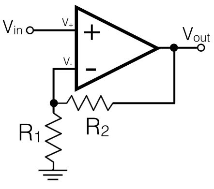
Rule 1 means high impedance. Rule 2 means that  $V_{out}$  relates to  $V_{in}=V_{+}=V_{-}$  through a simple voltage divider relationship:  $V_{-}=V_{out} R_{1}/(R_{1}+R_{2}) = V_{in}$ Solving for  $V_{out}$  in terms of  $V_{in}$  gives
