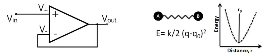
You can think of this as defining a potential distribution; deviations from equilibrium push the system back to equilibrium. Changing  $V_{in}$  changes the equilibrium point and the op-amp readjusts. Here the equilibrium is at  $V_{out} = V_{in}$ , which is r=0 in the spring analogy. We'll see how to adjust the equilibrium  $V_{out}(V_{in})$  relationship soon.
