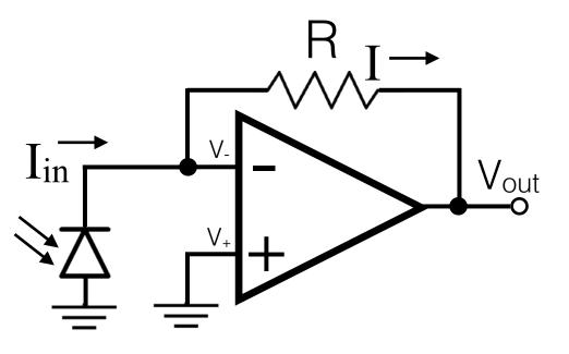
Rule 2 means V<sub>-</sub> = ground. Called a "virtual ground".
