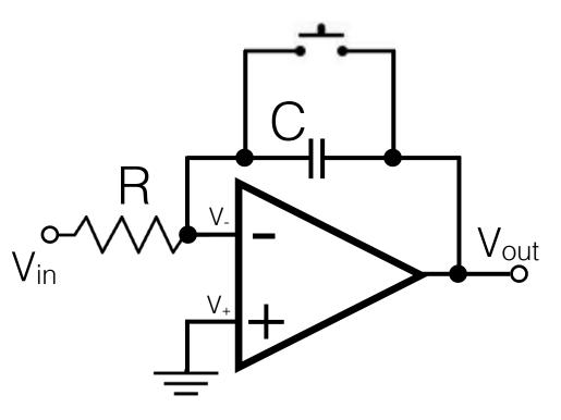
$V_{out}(t) = -(1/RC) \int V_{in}(t) dt$
