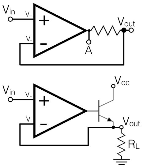
Rule 2 makes  $V_{out} = V_{in}$  regardless of any voltage dropped across the resistor.
