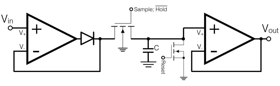
We can often time measurements, e.g., pump and probe. So we can use MOSFET switches from a control computer to time controls: reset, sample, hold, [readout], reset.
