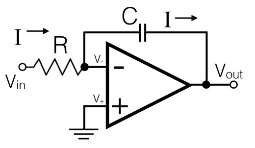
Using the golden rules we can analyze the circuit for an integrator
