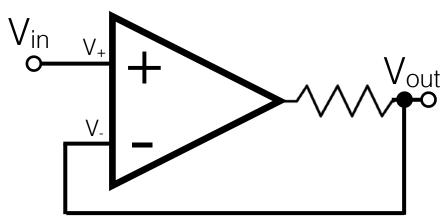
Rule 2 makes  $V_{out} = V_{in}$  regardless of any voltage dropped across the resistor.
