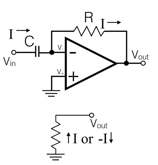
Rule 2 means  $V_{-}$  = ground. Called a "virtual ground".
