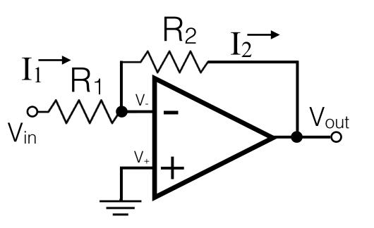
Rule 2 means  $V_-$  = ground. Called a "virtual ground".
