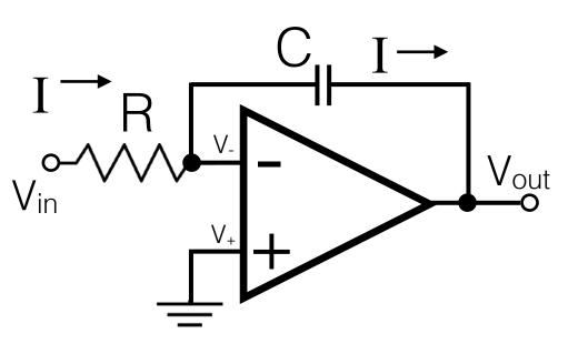
Rule 2 means  $V_-$  = ground. Called a "virtual ground".
