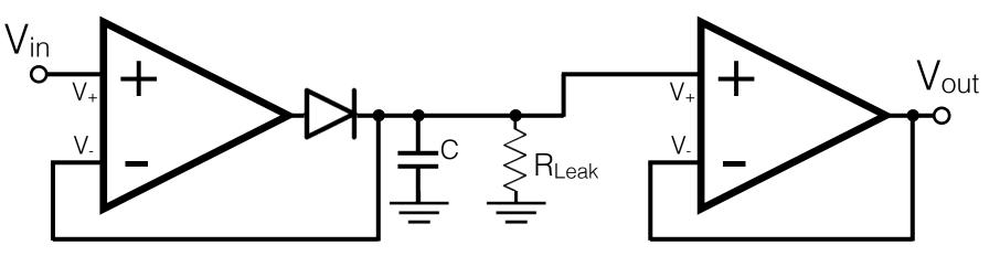
The output will follow on the way in The op-amp will compensate the di The diode won't let the op-amp pul The capacitor will hold the maximu The V<sub>-</sub> input will not allow current Can add a follower to avoid dischar Add a controlled resistor to leak of
