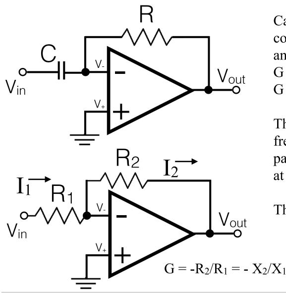
Can also think of this in terms of complex impedance, where it is an inverting amplifier with gain  $G = -X_R/X_C = -R/(-j/\omega C)$  $G = j\omega RC$
