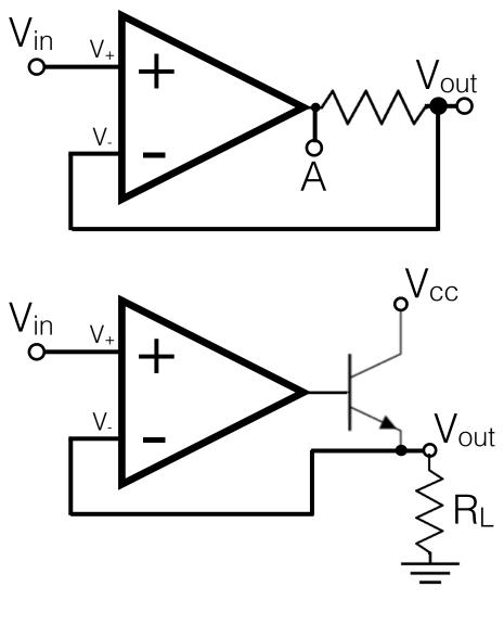
Rule 2 makes  $V_{out} = V_{in}$  regardless of any voltage dropped across the resistor.
