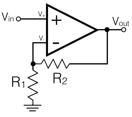
Rule 1 means high impedance. Rule 2 means that  $V_{out}$  relates to  $V_{in}=V_{+}=V_{-}$  through a simple voltage divider relationship.  $V_{-}=V_{out} R_{1}/(R_{1}+R_{2}) = V_{in}$
