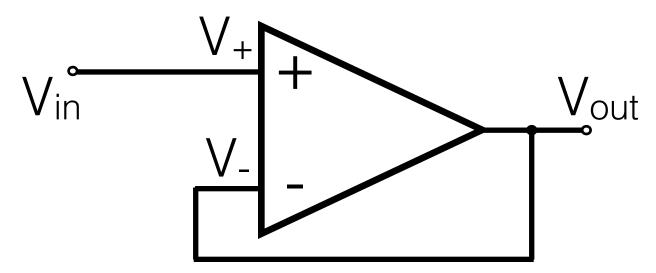
If  $V_{out} = V_{in}$  then  $V_+ = V_-$  and there is no difference to amplify, so no change. If  $V_{in} > V_{out}$  then  $V_+ > V_-$ , and that positive difference is strongly amplified to rapidly increase  $V_{out}$  until it reaches  $V_{in}$ .
