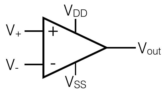
The external view of an op-amp is two inputs and one output, and power.
