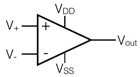
It operates as an enormous gain differential amplifier, so: if  $V_+ > V_-$  that difference is amplified to make  $V_{out} = V_{DD}$ . if  $V_+ < V_-$  that difference is amplified to make  $V_{out} = V_{SS}$ .
