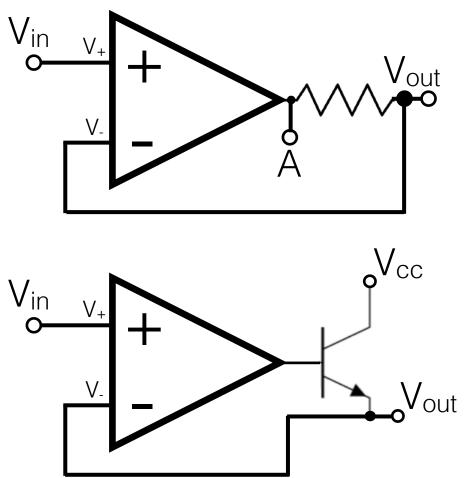
Rule 2 makes  $V_{out} = V_{in}$  regardless of any voltage dropped across the resistor.
