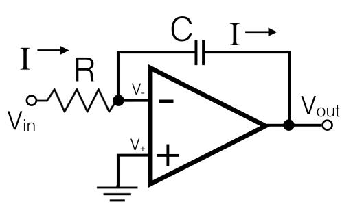
Rule 2 means V<sub>-</sub> = ground. Called a "virtual ground".
