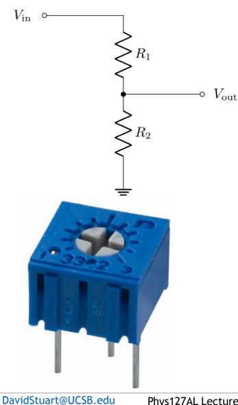
$$V_{out} = IR_2 = [V_{in}/(R_1 + R_2)] R_2$$
