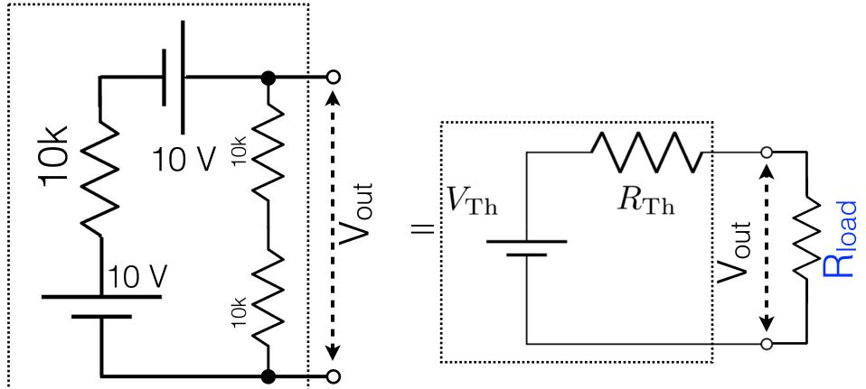
Any complicated mix of voltage sources & resistors can be treated as equivalent to this Thevenin equivalent circuit, i.e., it follows the same IV relation. That means if I attach *any value* of load resistor, R<sub>Load</sub>, across the terminals, the V<sub>out</sub> and I<sub>out</sub> will be the same between the two circuits, i.e., they're equivalent.
