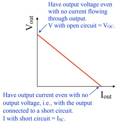
You can also find an equivalent circuit if we mix voltage sources and resistors
