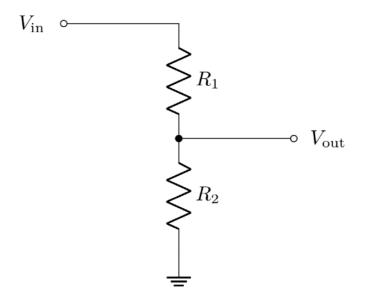
$$V_{out} = IR_2 = [V_{in}/(R_1 + R_2)] R_2$$
