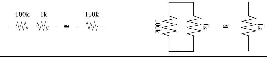
In series:  $R_T = R_1 + R_2$ . In parallel:  $1/R_T = 1/R_1 + 1/R_2 \implies R_T = R_1 R_2/(R_1 + R_2)$
