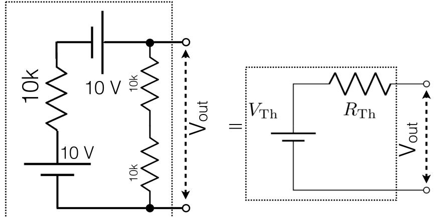
Any complicated mix of voltage sources & resistors can be treated as equivalent to this Thevenin equivalent circuit, i.e., it follows the same IV relation.
