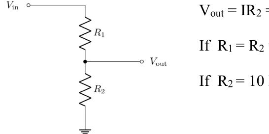
$$V_{out} = IR_2 = [V_{in}/(R_1 + R_2)] R_2$$
