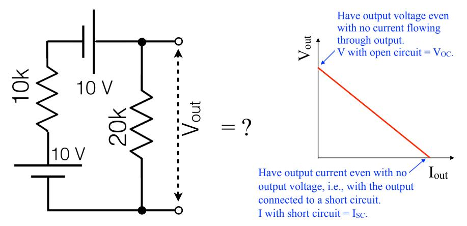
You can also find an equivalent circuit if we mix voltage sources and resistors
