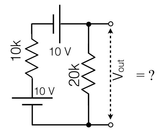
You can also find an equivalent circuit if we mix voltage sources and resistors
