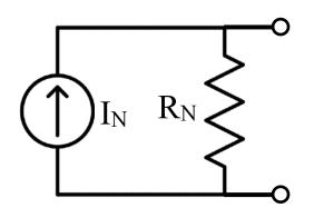
You would find  $I_N$  and  $R_N$  just as you found  $V_{Th}$  and  $R_{Th}$ . Consider the extreme load resistance options, 0 and infinity, and make sure that you get equivalent  $V_{out}$  and  $I_{out}$ .
