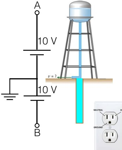
The idea of ground is to define a "zero point" of voltage for your circuit. This is arbitrary, but so it calling the ground's gravitational potential zero in U = mghAll that matters for energy is potential differences. All that matters for voltage is potential differences. So, pick a zero point for convenience.
