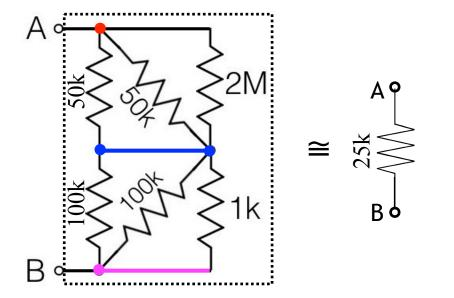
Any complicated mix of resistors can be treated as equivalent to a single resistor, which follows the same V = I R, i.e., the same IV relation.
