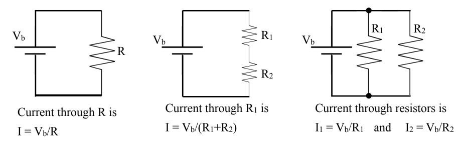
In series:  $R_T = R_1 + R_2$ . In parallel:  $1/R_T = 1/R_1 + 1/R_2 \implies R_T = R_1 R_2/(R_1 + R_2)$
