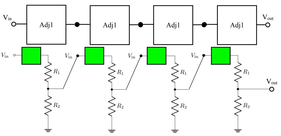
We need an "electromagical" impedance booster at the input of each stage We'll see how to do this soon, with a transistor.
