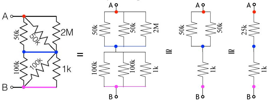
The open circles indicate terminals of the circuit, ie input/output points.
