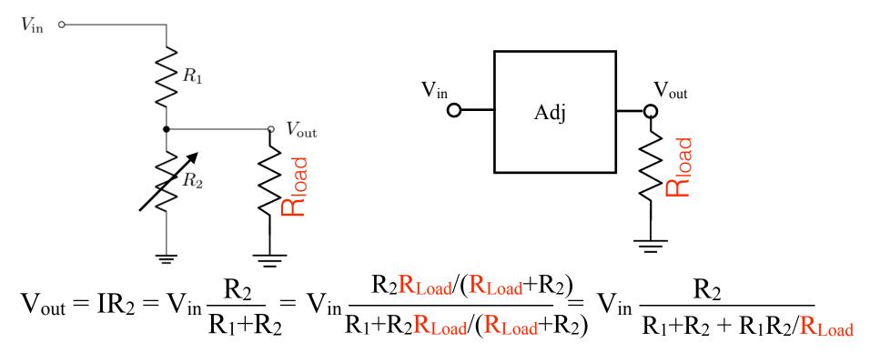
But, suppose I now connect this stage to the next stage in my circuit. In this case, it would be a lamp. That is the load.  $V_{out}$  is little changed by the load if  $R_{Load} \gg R_1 R_2/(R_1+R_2)$ .
